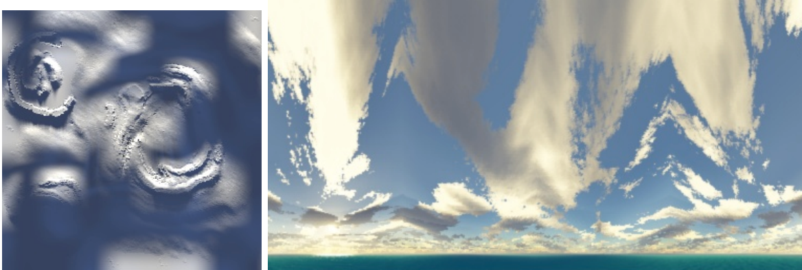
Fig. 3: A single frame of terrain lightmap and sky dome textures from a video based illumination map (VBIM) sequence.
